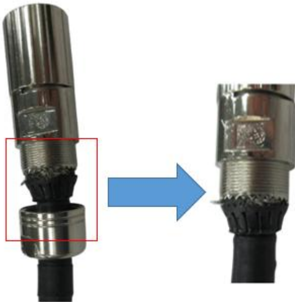
Fig.5 .17 : The shields must have a conductive connection to the circular connector
